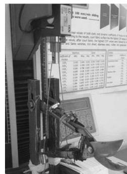
**Fig. 3** Lloyd instrument universal testing machine
