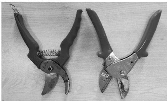
**Fig. 2** Bypass and Anvil type pruning shears
