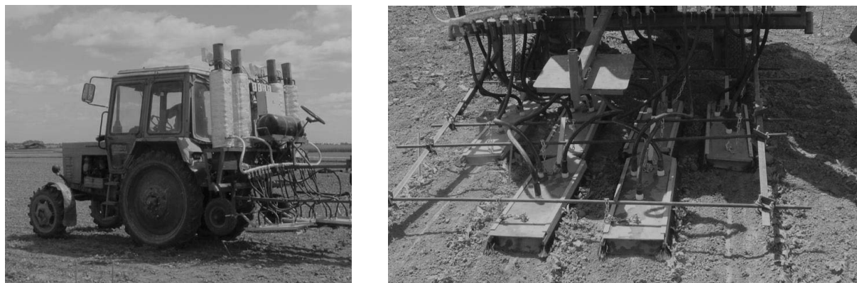
Fig. 1 Inter-row steaming machine
