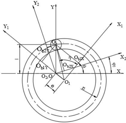
**Fig. 4** Generalized model of a groove cam
