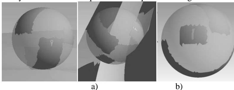
**Fig. 9** Cloud charts about contact pressure on the ball in contact with their grooves of the third design model a) the contact area with groove curve of the output shaft, b) the contact area with the groove of input camshaft, c) the contact area with the straight groove of the middle part
