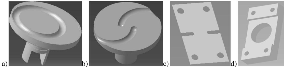
**Fig. 5** a) The shape of the input camshaft, b) the shape of the output shaft, c) the middle part, d) one of two frames of the groove cam mechanism for the second design model
