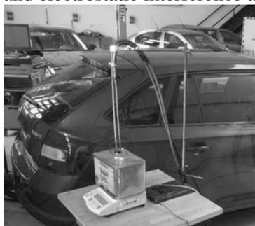
**Fig. 1** Connecting the scales to the vehicle
