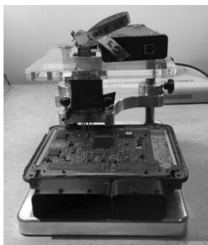
Fig. 2 The stand for the engine controller's software modification
