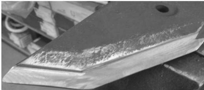
Fig. 1 Groove for hardfacing on the functional face part of the ploughshare point
