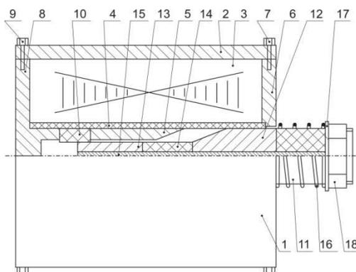
**Fig. 3** Linear electric motor: 1 is a stator; 2 is a magnetic body; 3 is a magnetizing coil; 4 is a non-magnetic frame; 5 is an upper magnetic pole; 6 is an end magnetic pole; 7 is a bolt; 8 is a lower magnetic pole; 9 is a bolt; 10 is a non-magnetic insert; 11 is an armature; 12 is an upper magnetic circuit of the armature; 13 is a bottom magnetic circuit of the armature; 14 is a non-magnetic bearing; 15 is a non-magnetic rod; 16 is a return spring; 17 is a washer; 18 is a nut
