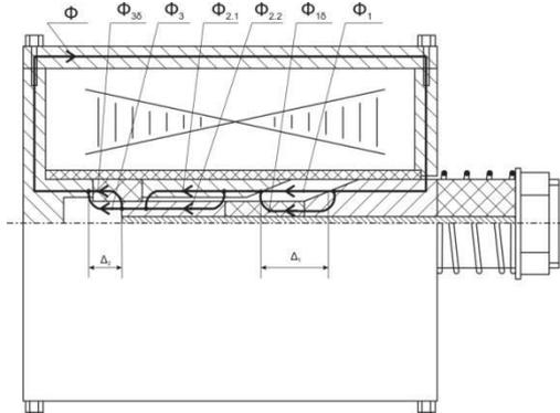
**Fig. 4** Magnetic fluxes of linear motor
